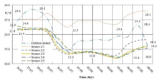
Fig. 5. Temperature °C, tank No.2 (with ozone), 26.07-08.08.2019
