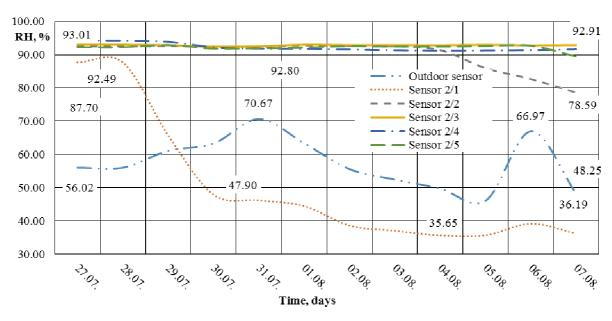
Fig. 3. Air humidity RH %, tank No. 2 (with ozone), 27.07-07.08.2019
