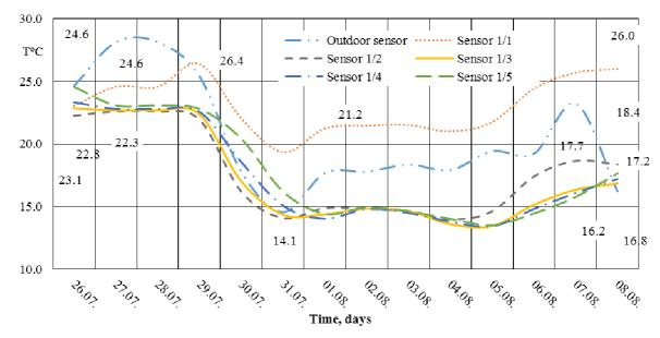
Fig. 4. Temperature °C, tank No.1 (without ozone), 26.07-08.08.2019
